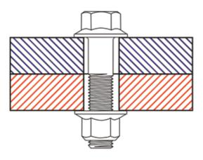
Figure 4: Top and Bottom Plates are Different Materials
