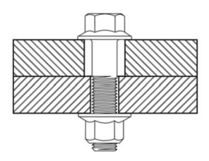
Figure 5: Top and Bottom Plates having Different Clearance Hole Diameters
