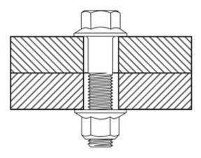
Figure 3: Top and Bottom Plates of the Same Material
