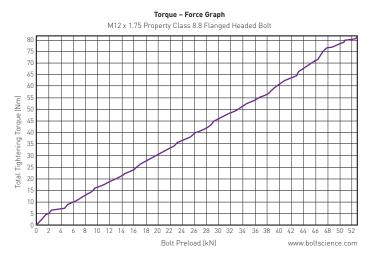
Figure 1: Torque – Tension Relationship
