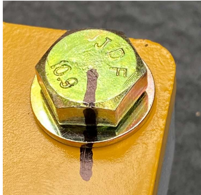
Torque Stripe Applied to Bolt Head (Bolt in Assembled in Tapped Hole)
